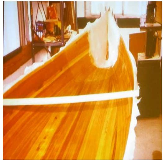
*First step after flipping: lots and lots of sanding. Then fiberglass using extra layer at bow.*
