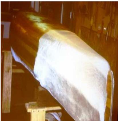
*Fiberglassing bow with 6-ounce material after using 4-ounce in the center area*
