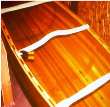
*After trimming the fiberglass, Jeff installs the gunnels, the carrying bar, the stern and bow decks, and the seats.*
